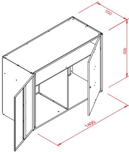
LES ARMOIRES À PNEUS ET ACCESSOIRES ASSOCIENT SÉCURITÉ ET ESTHÉTIQUE. SÉCURITÉ CAR ELLES SONT ANTI-FEU ET LEURS PORTES VERROUILLABLES: ELLES PROTÈGENT DES VOLS. LA STRUCTURE SOLIDE, EN TÔLE D'ACIER, EST ZINGUÉE. LE MODÈLE STANDARD SANS PAROI ARRIÈRE S'ADAPTE AU MONTAGE MURAL. AUSSI DISPONIBLE AVEC PAROI ARRIÈRE POUR POSE AU PLAFOND OU AU SOL.
