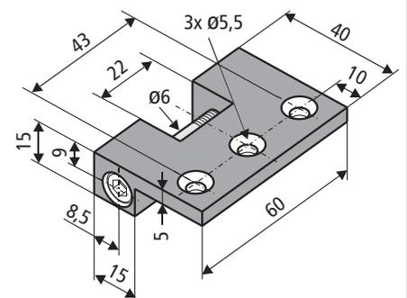
**ÉTAPE DE MONTAGE 4: SCHÉMA DE PERÇAGE POUR CONSOLE ET SUPPORT DE VANTAIL**
